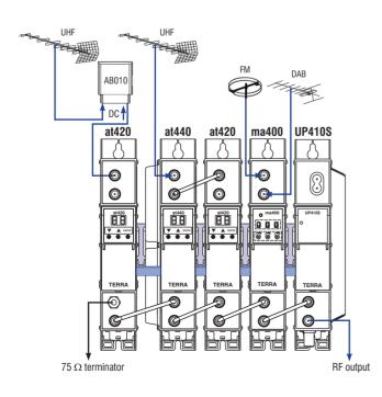
Application diagram of filtering 8 TV channels from 2 directions & combining with FM and DAB signals.
