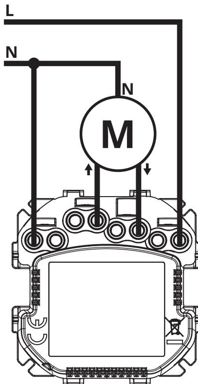
Diagram 1: Example connection with roller blind motor
