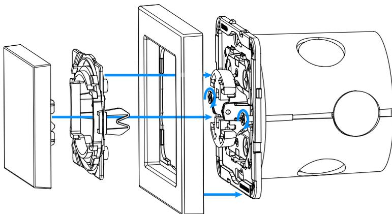
1. Insert the device with mounting frame into the mounting box and secure with mounting claws and screws.
