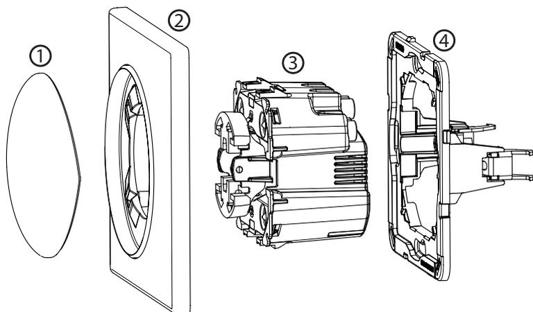
1 – switch button, 2 – cover plate, 3 – unit (device), 4 – mounting frame
