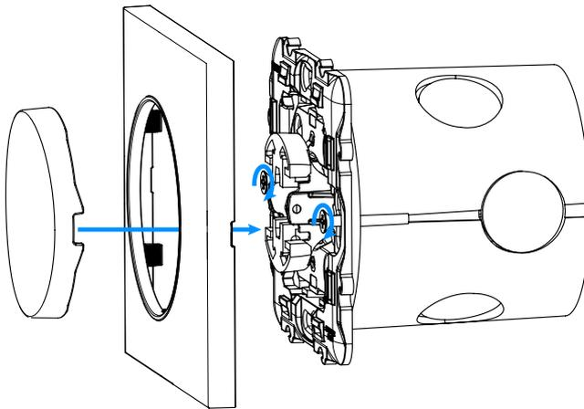
1. Insert the device with mounting frame\* into the mounting box and secure with mounting claws and screws.
