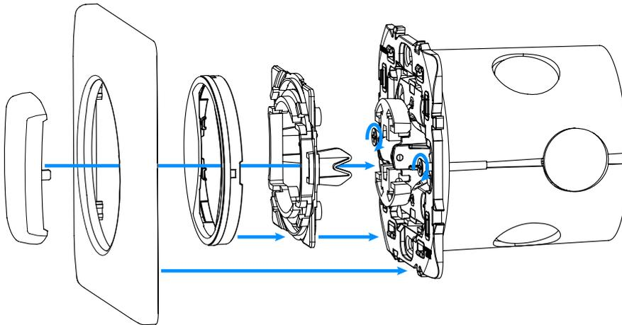
1. Insert the device with mounting frame\* into the mounting box and secure with mounting claws and screws.
