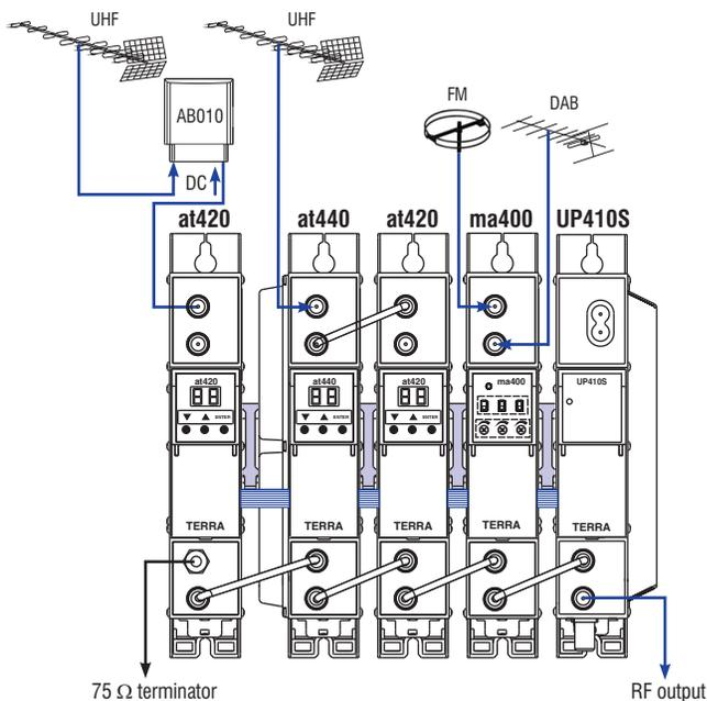
Application diagram of filtering 8 TV channels from 2 directions & combining with FM and DAB signals.
