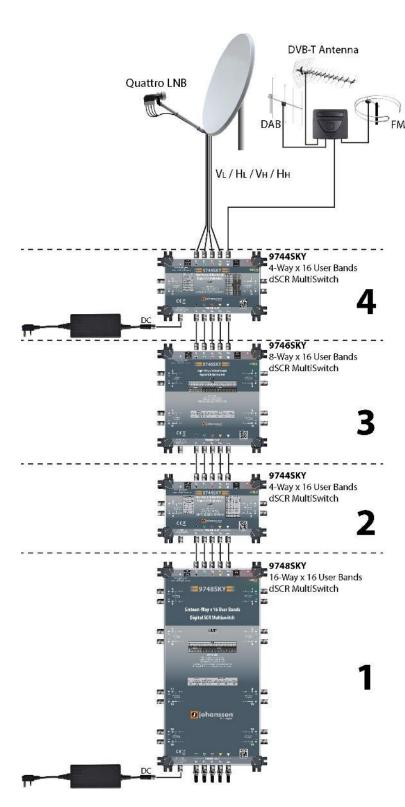
The optional power supply (ref 2460/2460UK) can feed multiple multiswitches.
