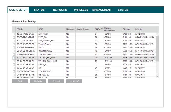
4. If the root AP needs password to be connected, you should select the same Mode, Channel Width and Security type and enter the same PSK Password as entered on the root AP. Enter the distance between this device and the root AP/router in Distance setting. Then click Next.
