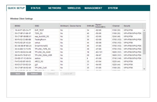
4. If the root AP needs password to be connected, you should select the same *Mode*, *Channel Width* and *Security* type and enter the same *PSK Password* as entered on the root AP/router. Enter the distance between this device and the root AP/router in *Distance setting*. Then click **Next**.
