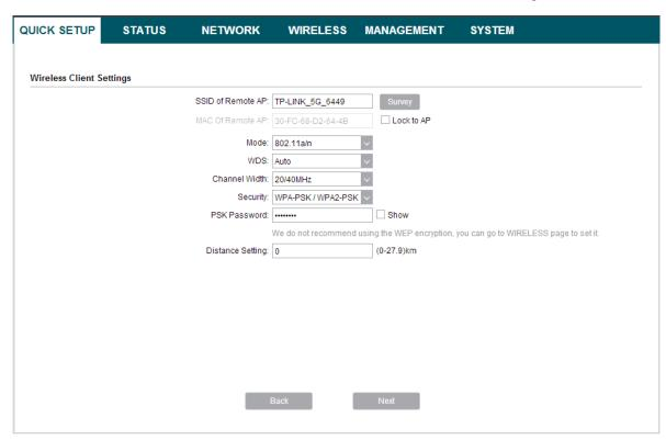
5. Create a new *SSID* and *PSK password* for the local wireless network. The wireless AP settings for the local network will be set the same as your root AP by default. Click **Next**.
