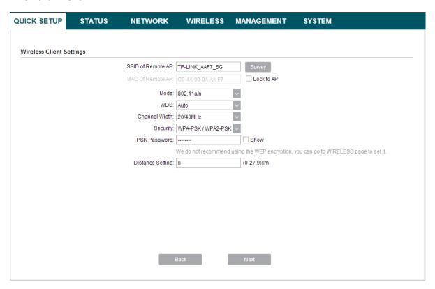
**6.** Create a new *SSID* and *PSK Password* for the local wireless network. The wireless AP settings for the local network will be set the same as your root AP by default. Click **Next**.
