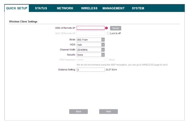
4. The AP list will appear as shown below. Select the desired wireless network and click Connect. It's possible that two or more networks use the same SSID in the AP list. Lock to AP can make the device connect to the specified AP you had connected before the next time.
