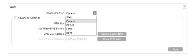
There are five WAN connection types: Static, Dynamic, PPPoE, L2TP, and PPTP. Select the suitable one to configure the IP parameters of the WAN on the screen below. If you are not sure of the connection type, please consult your ISP.
