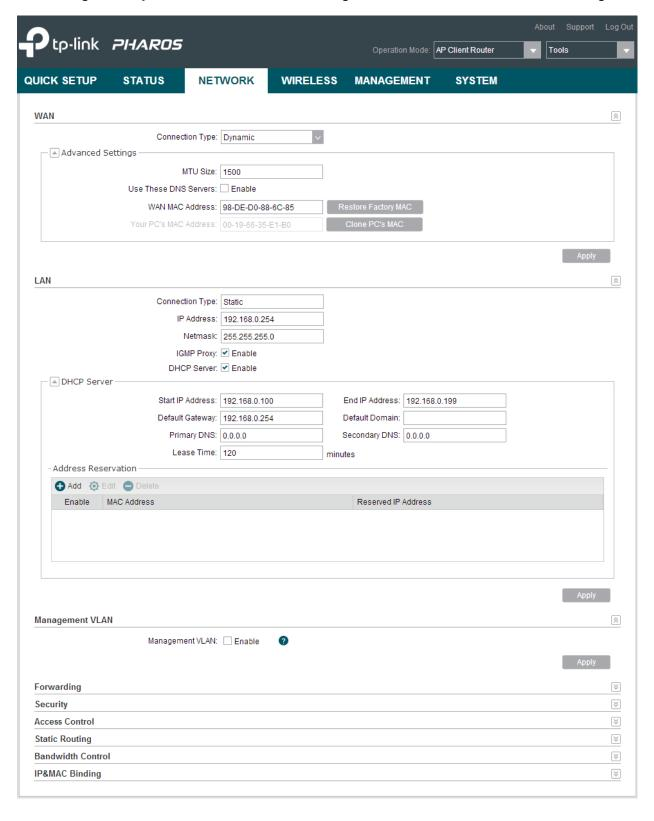
If you've made any change of the parameters, click **Apply** to make the configuration take effect. There will be a blue bar at the top of the page to remind you to save the configuration. Click **Save Changes** when you finish all settings, otherwise all the settings will be recovered to last saved settings at reboot or power off.
