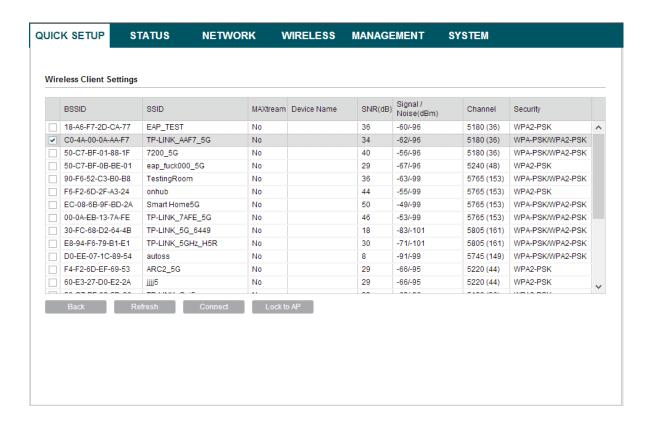
5. If the root AP needs password to be connected, you should select the same Mode, Channel Width and Security type and enter the same PSK Password as entered on the root AP/router. Enter the distance between this device and the root AP/router in Distance setting. Then click Next.
