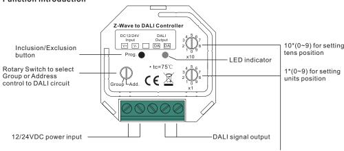
Rotary switches for setting DALI Group number (0-15) or Address number (0-63) to be controlled, the number equals to tens position plus units position
