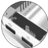
The end of line jumper is placed on the CN4 connector, that can be located on the monitor base. In case of twisted pair cable installations, the end of line jumper is placed in the EL562 module, also located in the CN4 connector of the monitor base.
